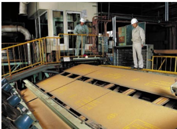
The trim saw process (cutting products to size). Inspectors visually check each board.
